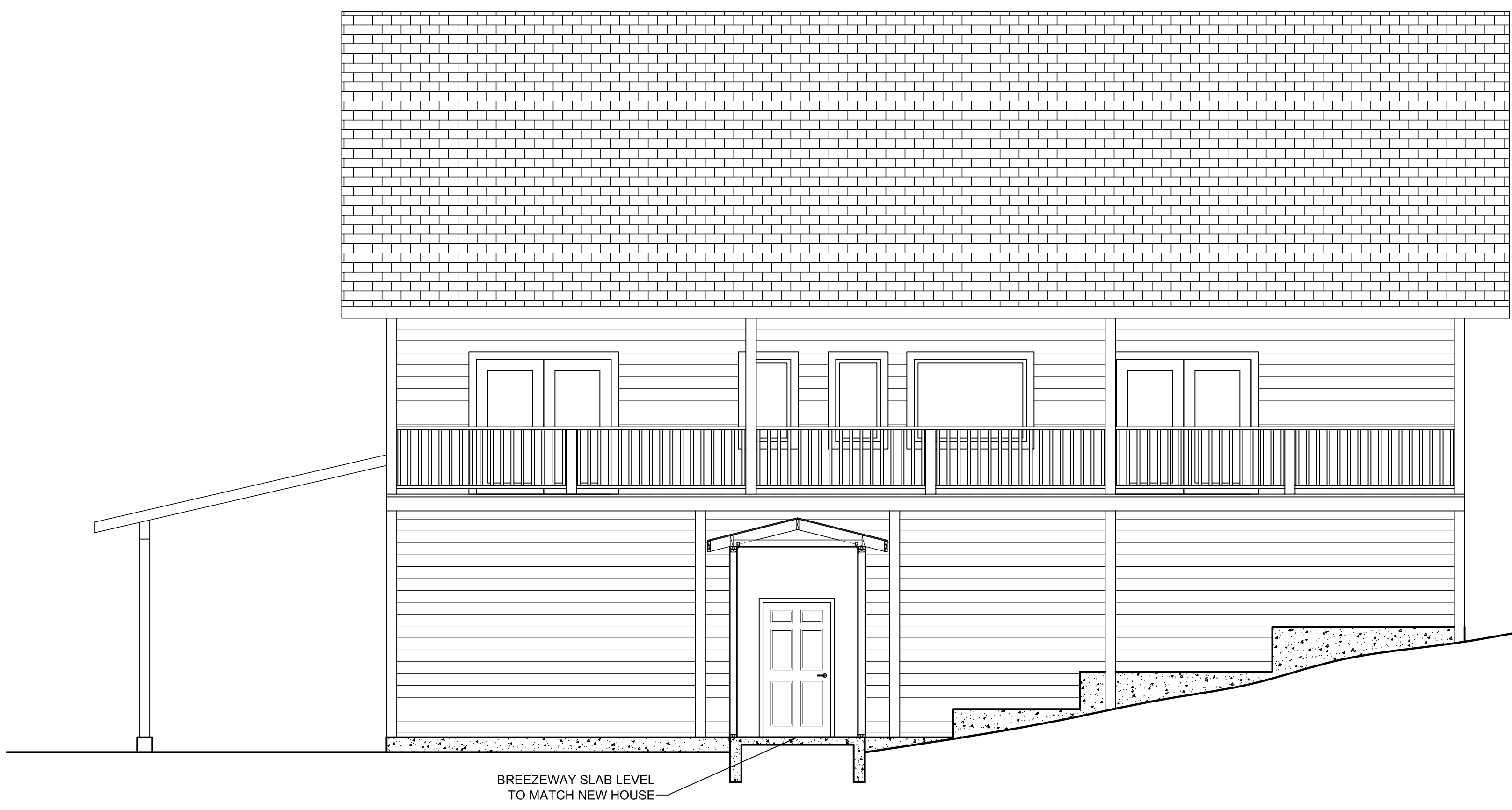
C-2 A1.1 NEW STRUCTURE, EAST ELEVATION SCALE: 1/4" = 1'-0"
